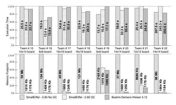
Figure 6: Execution time and memory footprint comparisons of leaky programs under UNIX
