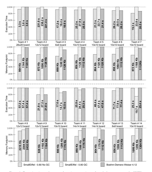
Figure 5: Execution time and memory footprint comparisons of non-leaky programs under UNIX
