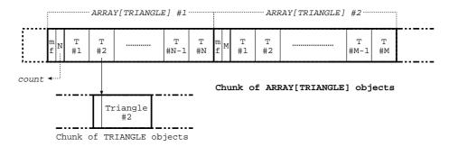
Figure 4: Detail of a resizable object chunk
