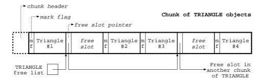
Figure 2: Detail of a fixed-size object chunk
